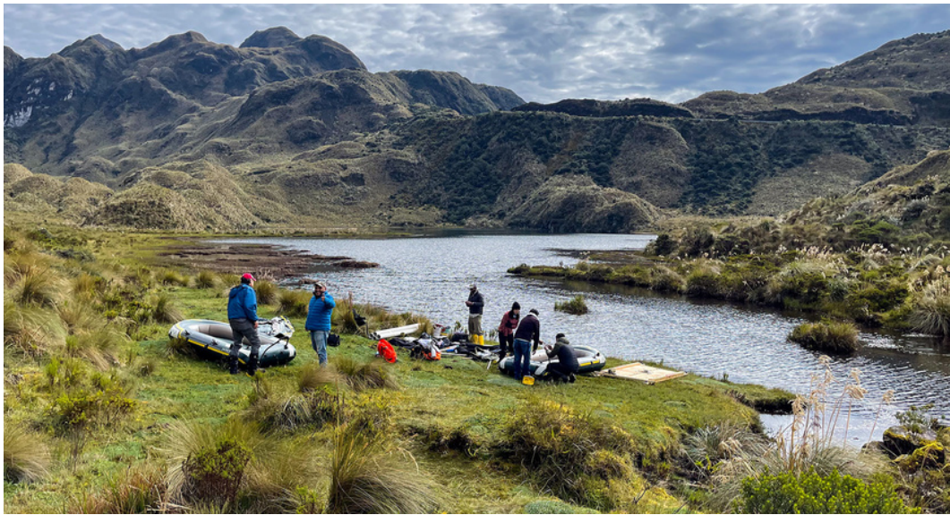
Team members inflate rafts and organize coring equipment on the shore of Laguna Kuyuk. One raft is used to anchor and stretch perpendicular ropes to secure the platform, which is suspended across two rafts.
